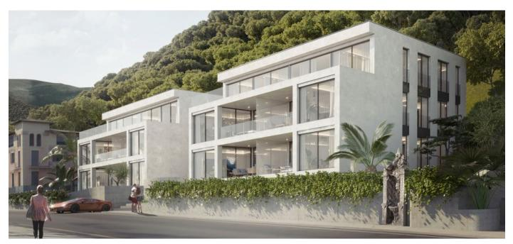
The project concerns the realisation of 2 buildings with 10 flats of different sizes and an underground parking; the total volume is 5600 m3. The housing complex oriented west is placed on a hill closed to the wood; for the excavation it was necessary to preview provisional retaining walls on a total surface of around 500 m2. The structure frame is in reinforced concrete with rectangular raster.
